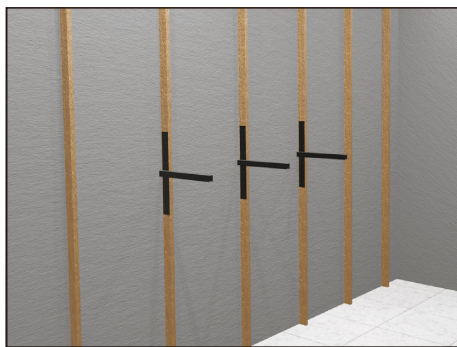
① Make sure the horizontal of each shelf bracket using the square pipe and fix to the core material
